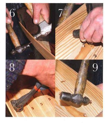
Driving nail through land using ball peen hammer outside and claw hammer inside to stop bounce
